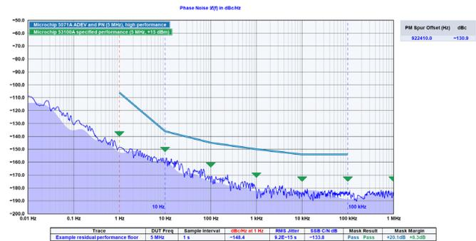
53100A phase noise test software is shipped along with the product. It allows a user to set up various measurement configurations/speeds, toggle display settings, import/export data, run scripts, set up mask lines and more. Visit [microchip.com/53100A](http://microchip.com/53100A) for more information.
