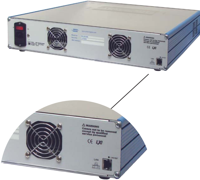
Fig. 3.5 - Detail showing the LAN Connection Socket and LAN Reset Switch on the back of the Pickering LXI High Voltage 2-Pole Matrix 60-310
