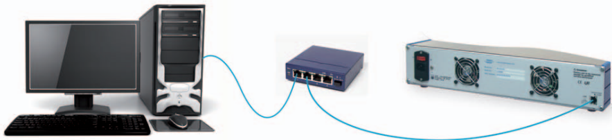
Fig. 2.2 - Connection to an LXI Device through a network device such as an Ethernet Switch
