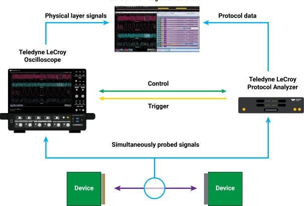
Interoperability issues can lead to finger-pointing exercises that cost money and delay time-to-market. *Cross*Sync PHY technology merges the functions of a Teledyne LeCroy oscilloscope with a PCI Express or USB protocol analyzer for insight into link behavior that no other instrument can provide.
