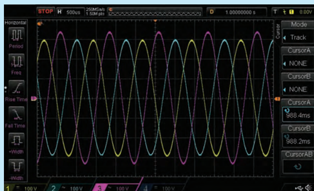
Three Phase Unbalance Voltage Test Captured
