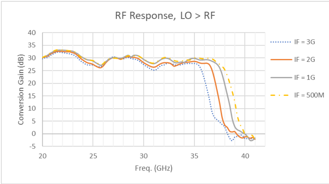
Figure 3. Measured conversion path RF response for different IF with LO > RF; If an external LO is used, the power is set at 5 dBm.
