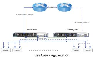
Accuracy is the relative offset between the active and standby units and is lower than 5 ns relative to the 1 PPS output on the active unit. A single IP management address is used. Health metrics and check mechanisms ensure proper monitoring of units to trigger the redundancy mechanism (switch over event). The redundancy schema is non-revertive. Manual intervention is required if the user decides to switch back to the original active unit once it is back in operation.
