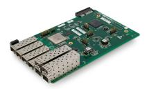
The 1 GbE/100 Mbps/10 GbE expansion module provides 1 GbE fanout and 10 GbE support. The module features four SFP and four SFP+ ports to enable a combination of four 100 Mbps Fast Ethernet and four 1 GbE ports, or eight 1 GbE ports, or a combination of four 1 GbE ports and four 10 GbE ports. As networks evolve, 10 GbE has become more prevalent, so this internal fanout capability is critical to connect to newer network elements.
