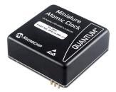
There are compelling reasons to use a Rubidium oscillator instead of an OCXO, but not all Rubidium oscillators are equal. Our miniature Rubidium clocks are available in a unique physics package based on the Coherent Population Trapping (CPT) atomic clock. These devices consume less power, operate over a wide range of temperature operations and have longer life cycles than legacy lamp-based Rubidium oscillators used in other products.
