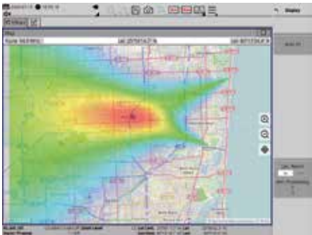
Script: Cooperative Bearing Several SignalSharks linked together via the Internet. One SignalShark takes over remote control of the others and receives the bearing results from them, which it combines as triangulations. This enables highly agile localization without the need for a central computer, with minimal outlay.
