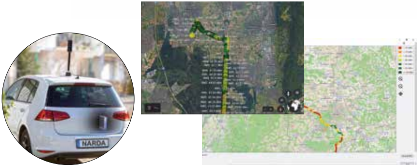
Script: Coverage Map The SignalShark synchronously records the level and position. These can be displayed as a coverage map on the internal map, or imported e.g. into Google Earth by exporting in *.kml format.
