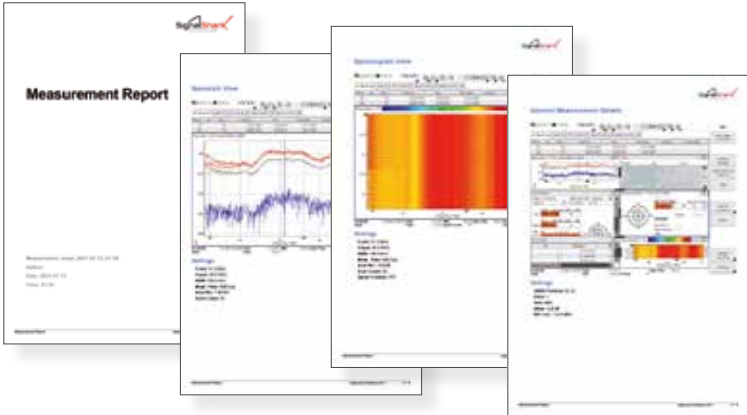
Script: Report Generator The Report Generator script maximises and creates a screenshot of each view in sequence and copies it along with the measurement settings into a user definable Word template.
