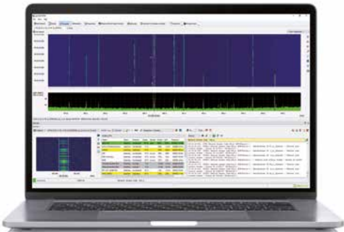
Example Procitec software Broadband signal displayed as a waterfall and a FFT spectrum Production of the selected narrow band signal, method detection and decoding mode Classification results: Decoder / Modem Decoding of contents starts after classification
