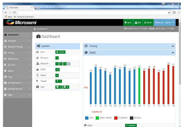
Track GPS/SBAS, GLONASS and/or BeiDou Satellite Constellations for improved integrity and satellite visibility in urban canyons.
